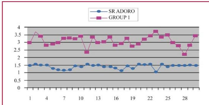
**Graph 1:** Wear measurements (mm) of 30 group 1 specimens (sintered alumina) compared with 30 SR ADORO® specimens ( $p < 0.05$ ). Wear measurements are shown on the vertical axis and specimen number along the horizontal axis.
