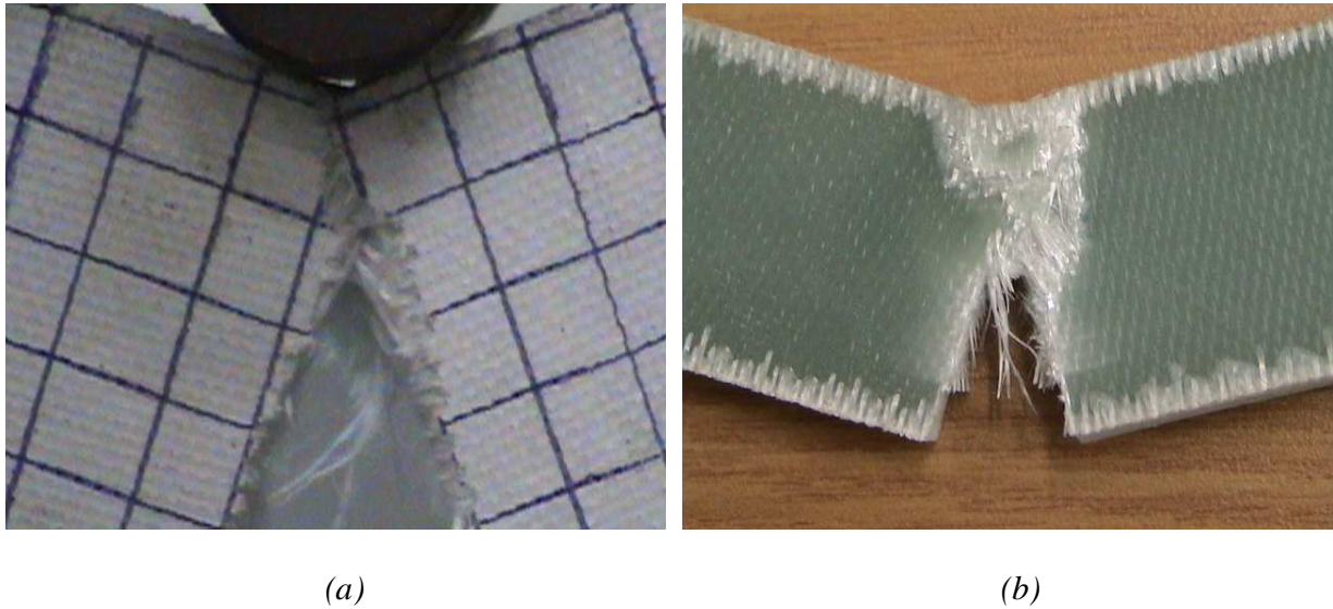
Figure 6.7: Fracture surfaces of Epoxy / Woven S2 Glass SENB test coupons showing (a) front of specimen, and (b) rear of specimen.
