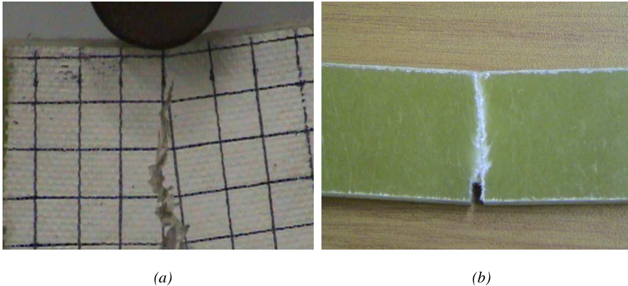
Figure 6.6: Fracture surfaces of Epoxy / Chopped S2 Glass SENB test coupons showing (a) front of specimen, and (b) rear of specimen.
