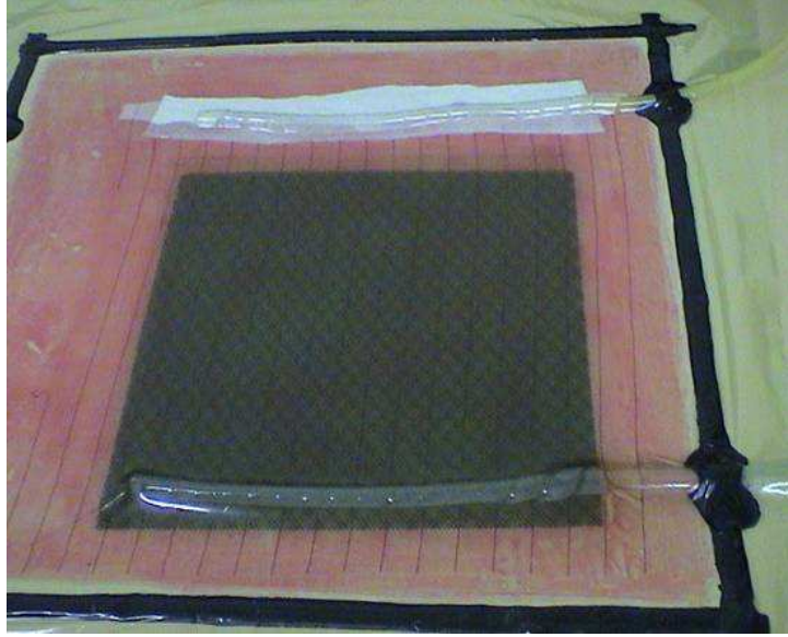
Figure 3.4: VARIM technique being used to manufacture a thermosetting panel
