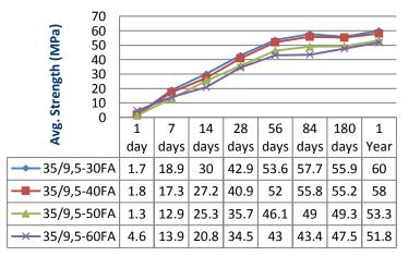
Figure 1: Compressive strength results of 35MPa mixtures
