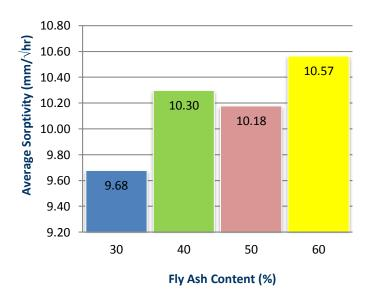
Figure 3. Water Sorptivity test results for the 35MPa concrete mixtures after 28 days
