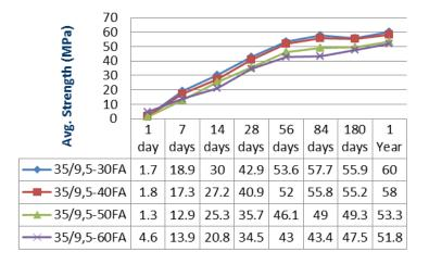
Figure 2: Compressive Strength results for the 35MPa concrete mixtures
