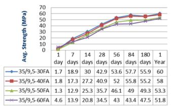
Figure 3: Compressive Strength results for the 50MPa concrete mixtures
