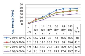
Figure 1: Compressive Strength results for the 25MPa concrete mixtures
