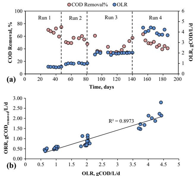
**Fig. 4.** (a) Time course of COD removal in the AnPBRR at different OLRs, and (b) organic removal rates (ORRs) versus OLRs.
