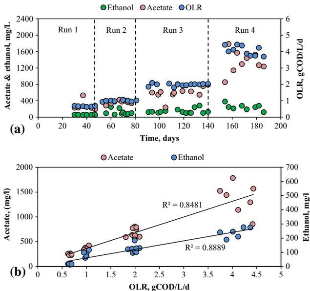
**Fig. 3.** (a) Time course of acetate and ethanol production versus OLRs, and (b) the relationship between acetate and ethanol generation at different OLRs.
