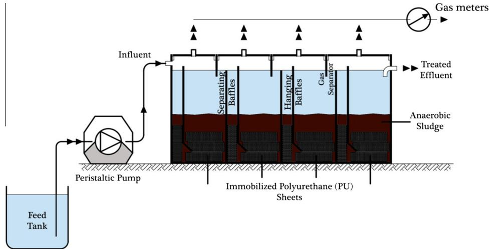
Fig. 1. Schematic diagram of the anaerobic packed bed baffled reactor (AnPBBR) for treatment of petrochemical industry wastewater.
