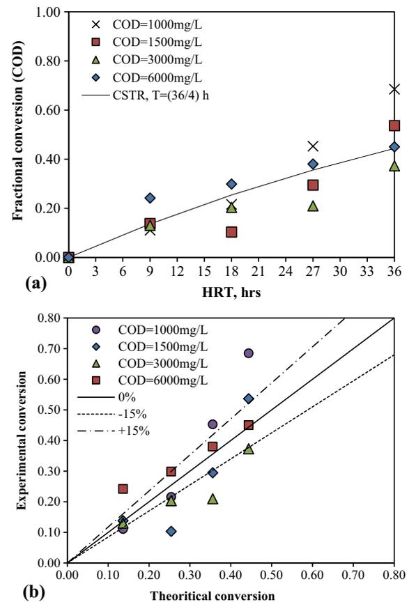
Fig. 6. (a) Experimental and theoretical fractional conversion (CSTR in series model) results' variation at each compartment with changing the initial COD, and (b) evaluation of the model versus experimental results.
