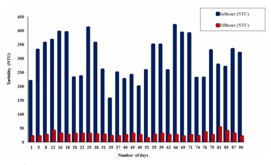
Figure 2 | Greywater influent and effluent turbidity over the 90 days of operation of the horizontal roughing filtration system at a constant filtration rate of 0.3 m/hr.
