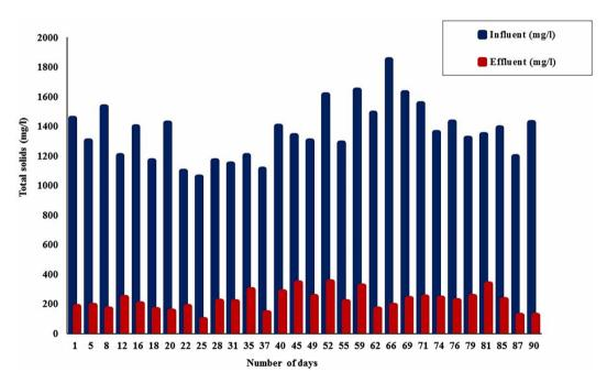
Figure 5 | Greywater influent and effluent total solids over the 90 days operation of the horizontal roughing filtration system at a constant filtration rate of 0.3 m/hr.
