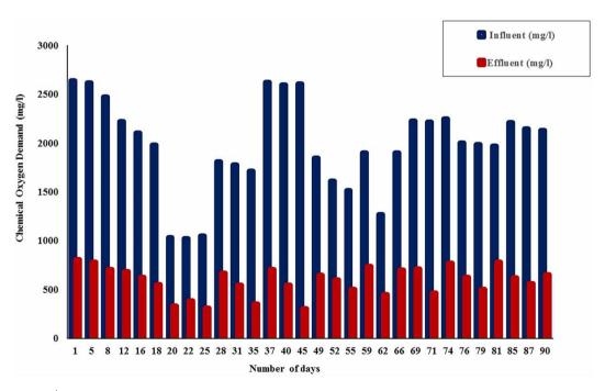
Figure 3 Greywater influent and effluent COD over the 90 days of operation of the horizonal roughing filtration system at a constant filtration rate of 0.3 m/hr.
