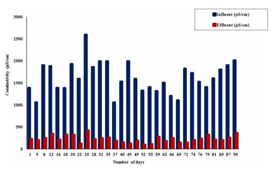
Figure 4 | Greywater influent and effluent conductivity over the 90 days of operation of the horizontal roughing filtration system at a constant filtration rate of 0.3 m/hr.
