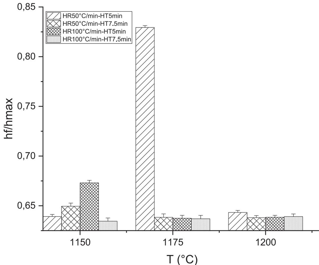
Fig. 5. Depth dependence ratio for as-sintered TiAl alloys for load of 100mN.
