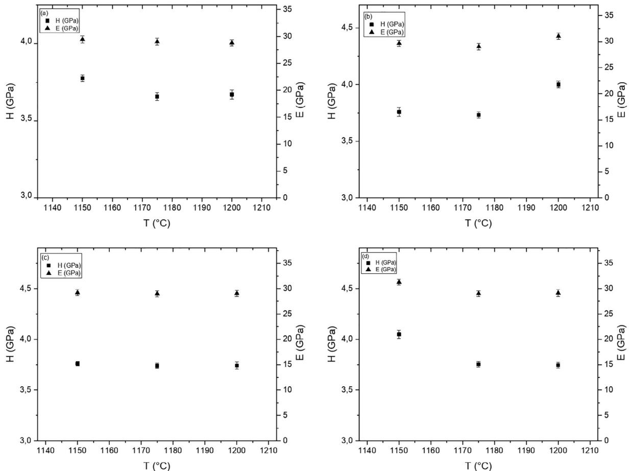
Fig. 4. Nanoindentation hardness and elastic modulus of the as-sintered TiAl alloys, sintered at 1150 °C, 1175 °C and 1200 °C, (a) with heating rate of 50 °C/min and holding time of 5 min, (b) with heating rate of 50 °C/min and holding time of 7.5 min, (c) with heating rate of 100 °C/min and holding time of 5 min, (d) with heating rate of 100 °C/min and holding time of 7.5 min.
