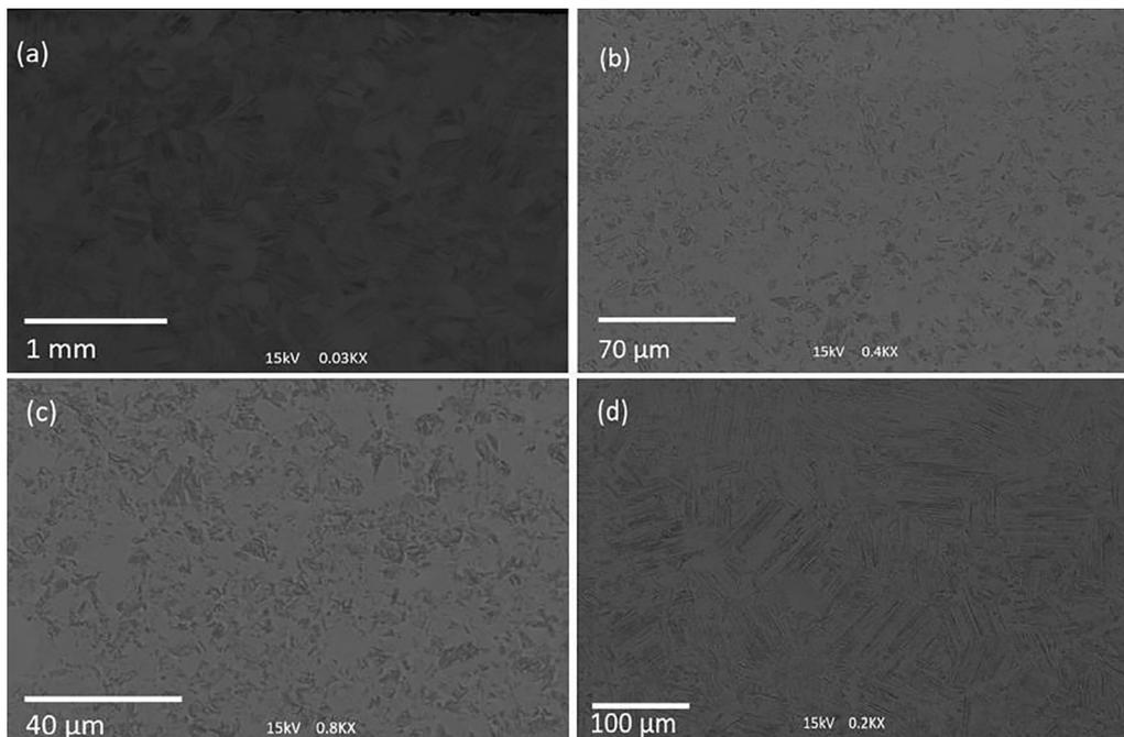
**Fig. 1.** SEM back scattered electron image of TiAl alloy sintered at, (a) T1150°C-50 MPa-HT5min-HR50°C/min (sample A), (b) T1175°C- 50 MPa-HT5min-HR100°C/min (sample H), (c) T1175°C-50 MPa-HT7.5 min-HR100°C/min (sample K), (d) T1200°C-50 MPa-HT7.5 min- HR50°C/min (sample F).
