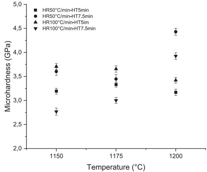
**Fig. 2.** Microhardness of the as-sintered TiAl, sintered at 1150 °C, 1175 °C and 1200 °C, with varied heating rate and holding time.
