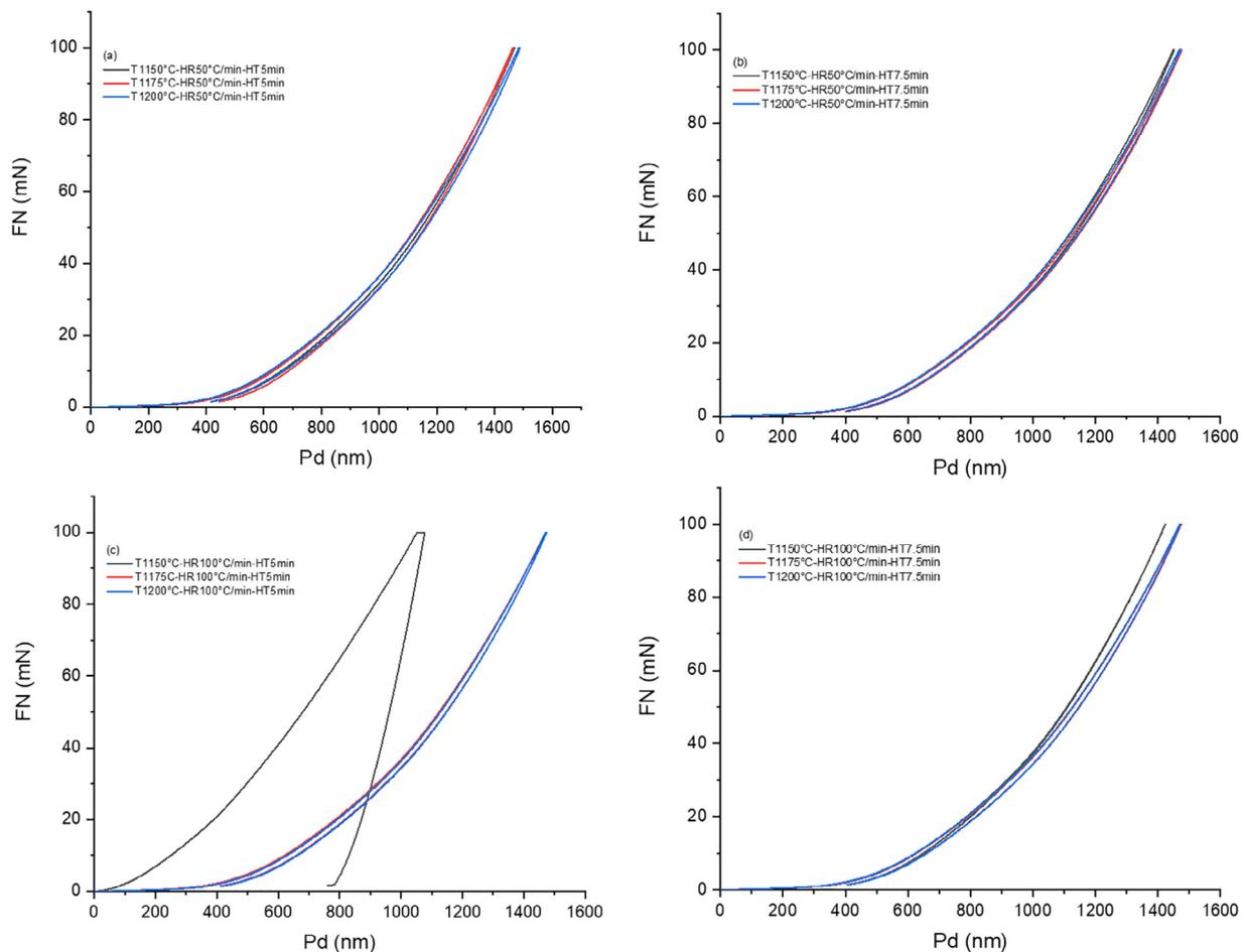
**Fig. 3.** Load-displacement curves of the TiAl alloys sintered at 1150 °C, 1175 °C and 1200 °C, (a) with heating rate of 50 °C/min and holding time of 5 min, (b) with heating rate of 50 °C/min and holding time of 7.5 min, (c) with heating rate of 100 °C/min and holding time of 5 min, (d) with heating rate of 100 °C/min and holding time of 7.5 min.
