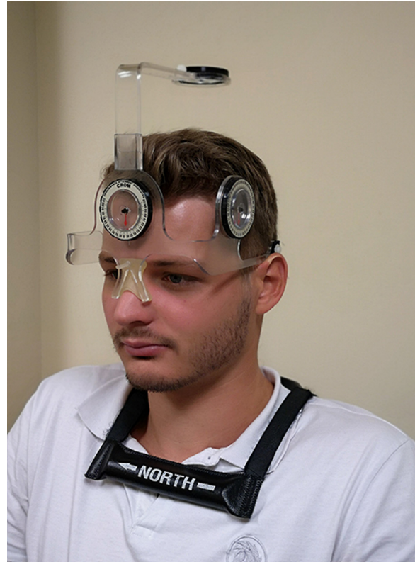
Fig 1. Cervical range of motion goniometer.
