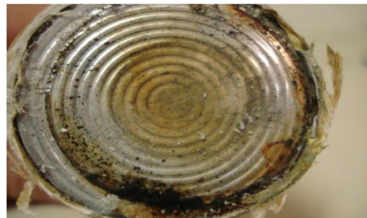
Figure 6. Moisture ingress on the sealing interior [16].
