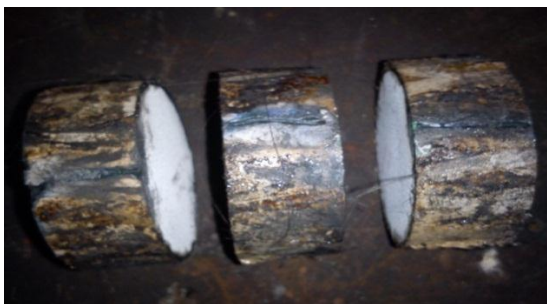
Figure 17. Cracks and damp on zinc oxide blocks.
