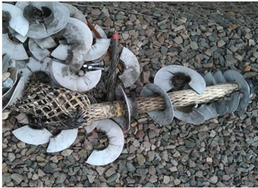
Figure 7. Metal oxide surge arresters with polymer housing that failed during in service condition.
