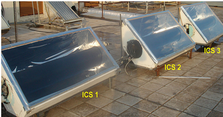
Fig. 6 Experimental CPC ICS models mounted at the test field [87]
