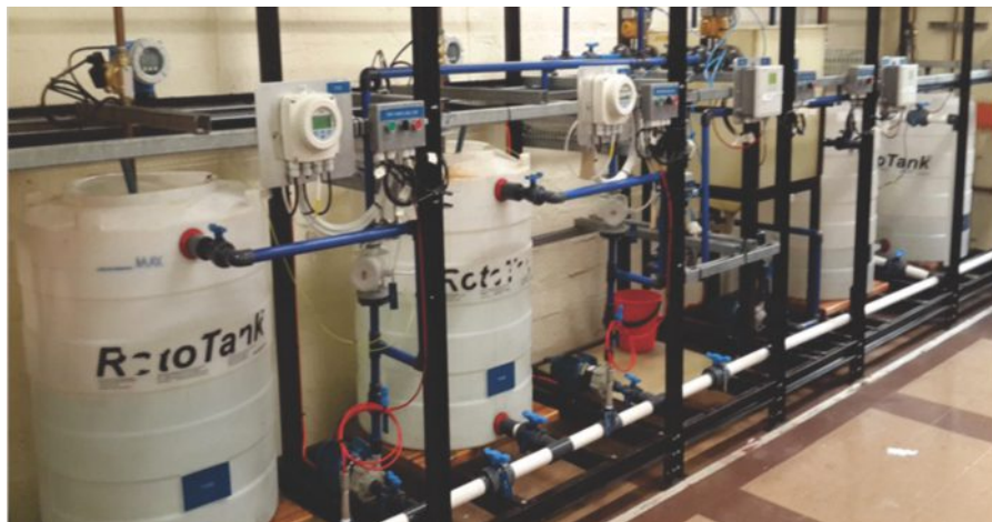
Figure 5. pH neutralization pilot plant housed in the Unit Optimization Studies Laboratory at the Durban University of Technology.
