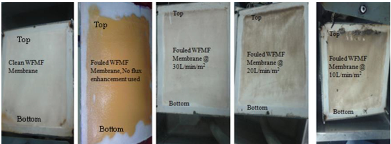
Fig. 6. Photos of fouled membranes at different aeration rates, the second membrane from the left is a fouled membrane without aeration.
