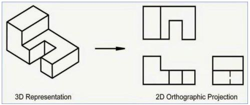
The above figure 1 shows 2d which is normally given to learners to manipulate and get the final product which is a 3d. The above figure is exactly in the way Sullivan (1964, p. 3) explains isometric drawing which is a conventionalized method of representing an object pictorially
