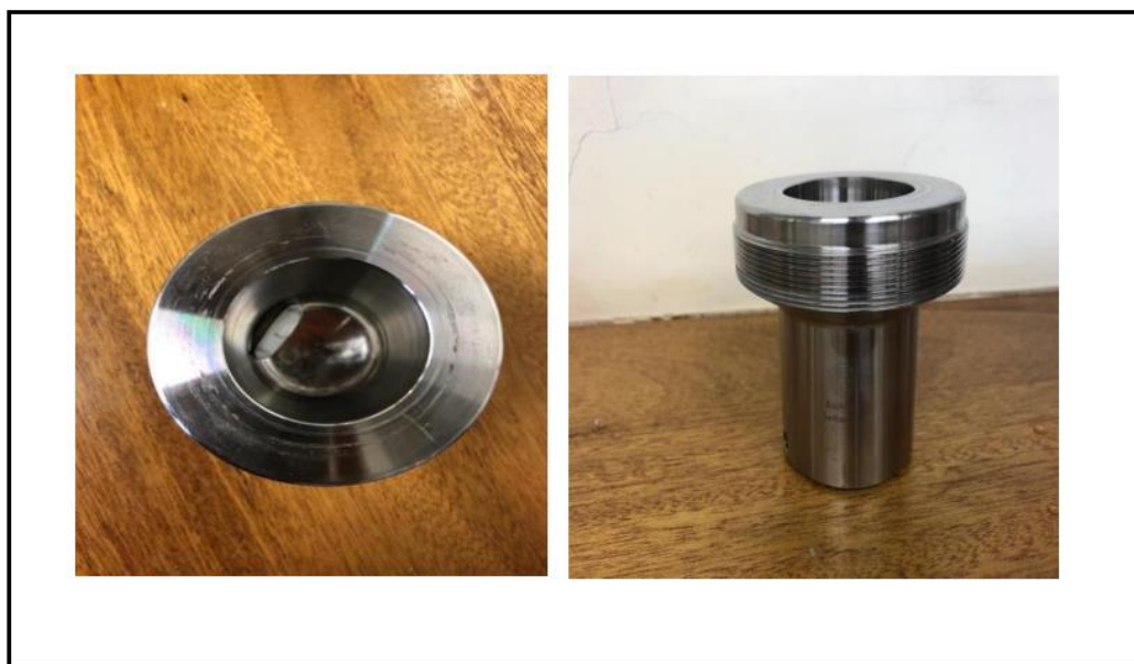
Figure 4-5: The top view of the equilibrium cell with magnetic stirrer inside, the picture on sideview of the cell.
