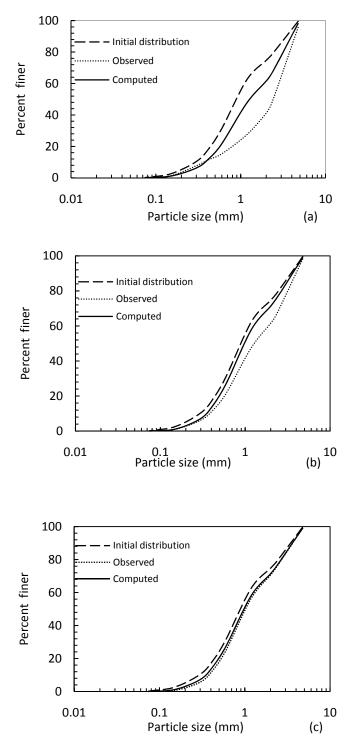
Fig. 2 Bed sorting for Run # at weir height: (a) Run 7, 10mm (Q =  $6.7m^3/h$ ); (b) Run 5, 15mm (Q =  $7.2m^3/s$ ); and (c) Run 3, 15mm (Q =  $8.1m^3/s$ )
